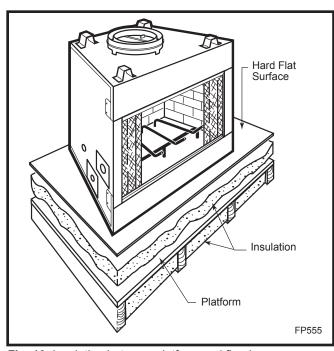
Fig. 10 Insulating between platform and fireplace.
